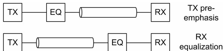
Fig. 11. Transmit (TX) pre-emphasis versus receiver (RX) equalization.
