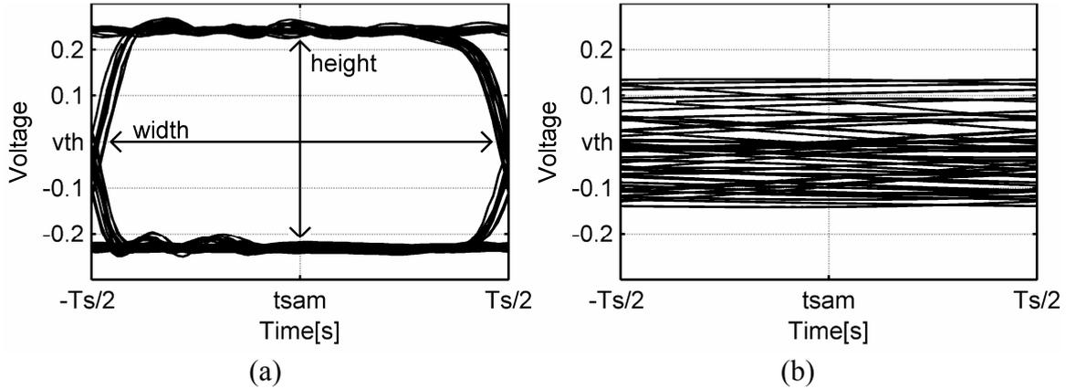
Fig. 9. Eye diagrams of measurements on 25m RG-58CU coaxial cable ( $R=5\text{Gb/s}$ ,  $T_s=200\text{ps}$ ).
